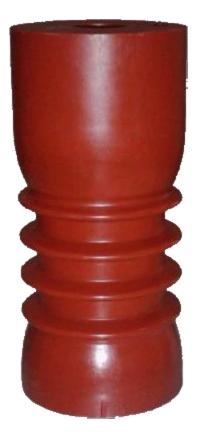
15KV Epoxy Insulator PG-4980 Height- 150mm Diameter- 69mm Creepage Distance- 182mm
